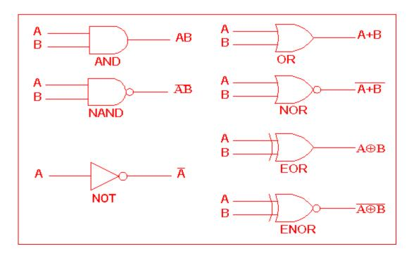
Table 2 is a summary truth table of the input/output combinations for the NOT gate together with all possible input/output combinations for the other gate functions. Also note that a truth table with 'n' inputs has 2<sup>n</sup> rows. You can compare the outputs of different gates.
