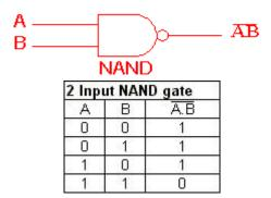
This is a NOT-AND gate which is equal to an AND gate followed by a NOT gate. The outputs of all NAND gates are high if **any** of the inputs are low. The symbol is an AND gate with a small circle on the output. The small circle represents inversion.
