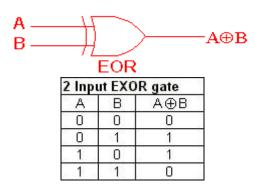
The 'Exclusive-OR' gate is a circuit which will give a high output if either, but not both, of its two inputs are high. An encircled plus sign (⊕) is used to show the EOR operation.
