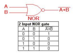
This is a NOT-OR gate which is equal to an OR gate followed by a NOT gate. The outputs of all NOR gates are low if **any** of the inputs are high. The symbol is an OR gate with a small circle on the output. The small circle represents inversion.
