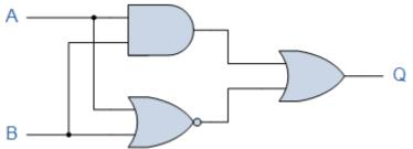
The system consists of an AND Gate, a NOR Gate and finally an OR Gate. The expression for the AND gate is A.B, and the expression for the NOR gate is A+B. Both these expressions are also separate inputs to the OR gate which is defined as A+B. Thus the final output expression is given as:
