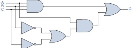
This system may look more complicated than the other two to analyse but again, the logic circuit just consists of simple AND, OR and NOT gates connected together.
