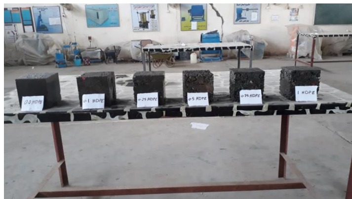
Figure 2: Concrete with pieces polyethylene waste after mixing.
