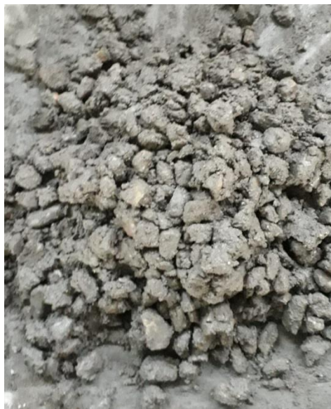
Figure 2: Concrete with pieces polyethylene waste after mixing.
