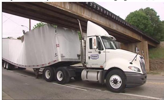
Figure 1. The laterally impact load with bridge girders
